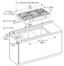
Minimum distance from the appliance out out to the side wall 11 (300 mm
