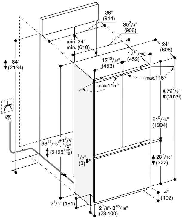
The door face dimensions are designed for a maximum gap of  $\frac{1}{8}$ " (3 mm).
